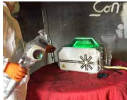
Figure 2: The 100 W Compact laser. Transparent film was wrapped around the laser and fibre delivery cable to protect them from the soot.
