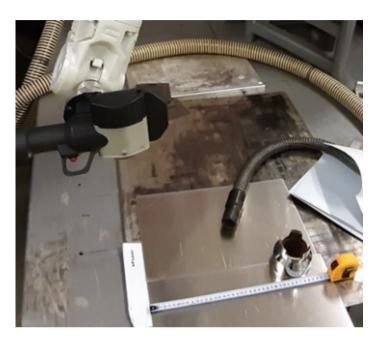
In the pictures above and below you can see the results of laser cleaning prior to welding. We used a QF-100 mounted on an ABB robot. Successful cleaning of Al oxide is shown at a cleaning travel speed of 2 m/min. with a focal distance of 300 mm.
