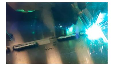
The photos above and below show MIG welding on the laserprepared aluminum at 5083°C. Different welding setups are used using ESAB MIG welding converters. Argon gas is used as shielding. Excessive welding spatter and welding fumes are observed on the surface if the surface has not been previously cleaned with the laser. Less smoke and spatter are observed on the laser-prepared Al surface during MIG welding.
